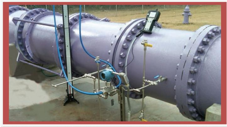
**HVT-PS insert meter with manual tap cleanout rods installed during field calibration of DP transmitter with manometer and hand-held programmer.**
